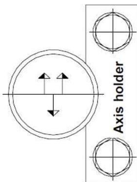
By means of an **Axis holder** which engages the milled nut of one of the outer bearings either *horizontally, vertically, from the left or from the right*, the axis must be fixed and secured in an axial and a radial direction.
