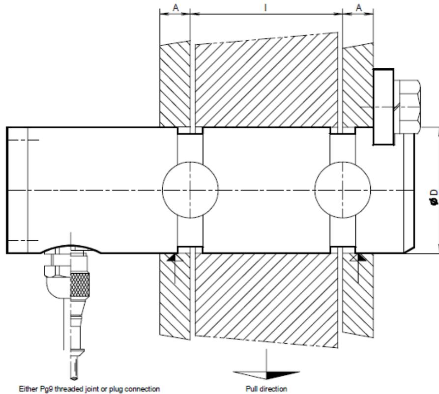
The Load Pin must be embedded in a smooth running but free of mechanical play in the inner bearing and lubricated. If the Load Pin is equipped with lubricating nuts or drill holes, maintenance must be carried out at regular intervals.
